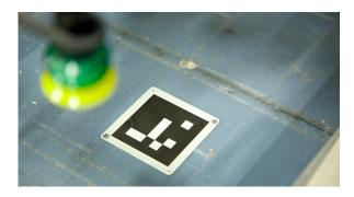
BAXTER ADAPTS QUICKLY TO WORKSTATION CHANGES OF UP TO +/-50MM HORIZONTALLY AND WITHIN +/- 10 DEGREES OF ROTATION.
